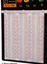
breadboard mounted on a metal plate. complete with four terminals. Note the numbered columns and lettered rows plus the ten supply rail rows, marked by red and blue lines. Available from Altronics (Cat PP1015A; \$47.95) www.altronics.com.au.
