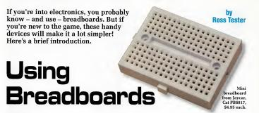
These days, 99% of electronics projects are soldered onto PCBs, or Printed Circuit Boards. But for experimentation, circuit development and "proof of concept" (ie, does it work!), nothing beats a solder-less breadboard (sometimes called a prototyping board).
